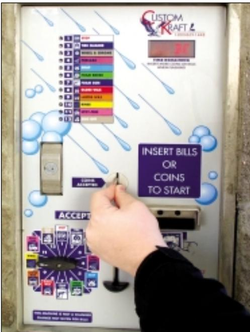
**Left:** Test each bay meter by inserting coin, token, credit card, and/or bill as applicable.
